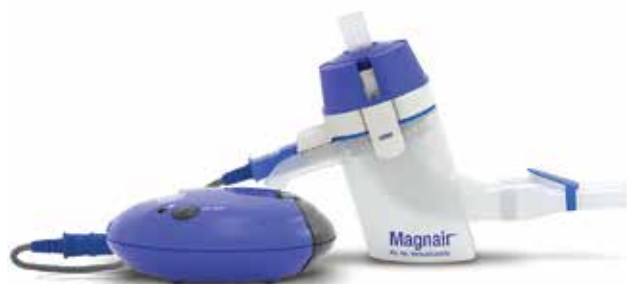
Figure 9. The Magnair is a vibrating mesh nebulizer (With permission from Sunovion)
