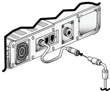
While the ventilator is plugged in, the internal battery is continuously charged.
