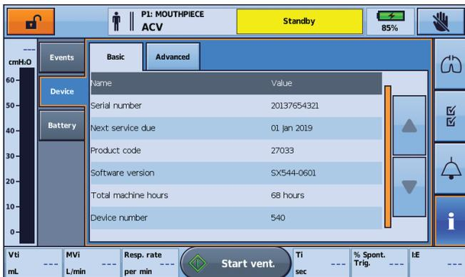
Locate the serial number and software version on the updated device screen.
