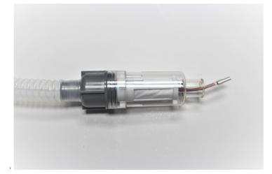
The unique coaxial design of the Proxima heated humidifier allows for true patientproximal heated humidification via the lowvoltage miniaturized heater core. The heater is in the center of the flow, but surrounded by a .2 micron filter that allows only pure, sterile water vapor into the gas stream.
