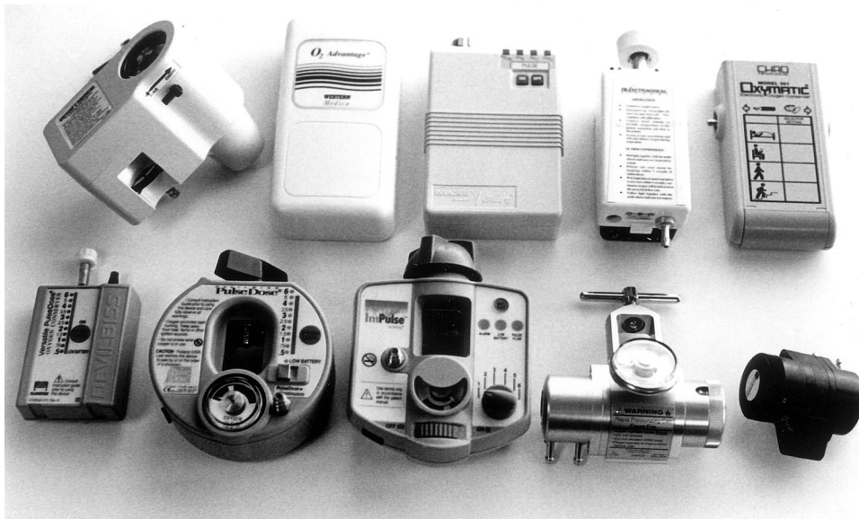
Fig. 5. Intermittent-flow oxygen-conserving devices. Front row (left to right): EX-3000 (DeVilbiss, Somerset, Pennsylvania), EX-2000 (DeVilbiss), Impulse Select (AirSep, Buffalo, New York), CR-50 (Mallinckrodt, St Louis, Missouri) OxiClip (Mallinckrodt). Back row (left to right): O 2 N Demand (Victor, Denton, Texas), O 2 Advantage (Western Medica, Westlake, Ohio), Venture (Invacare, Elyria, Ohio), DOC-2000 (Transtracheal Systems, Englewood, Colorado), Oxymatic 301 (Chad Therapeutics, Chatsworth, California).
